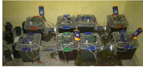
Fig. 2. A complete set up of a microbial fuel cell using carbon electrodes.
