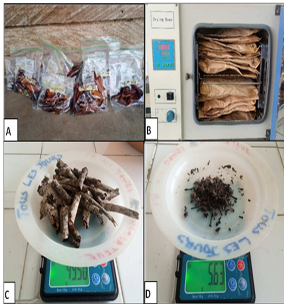
Fig. 3. Litterfall treatments: A. Collection of samples in the field, B. Oven drying, C. Twigs weighing, D. Flowers weighing
