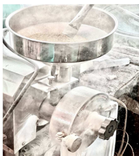
f. Commercial miller for pulverizing dried Gracilaria
