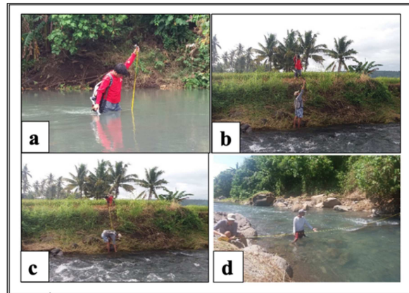
Fig. 2. Field Measurements on the study area; a) river stage at base flow b) bank height c) bank face length and d) channel width
