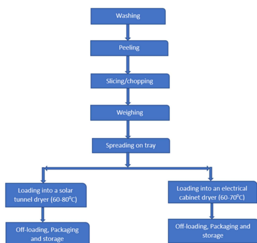
Fig. 1. General flow diagram for fruit drying (Modified from King'ori et al. , 1999)
