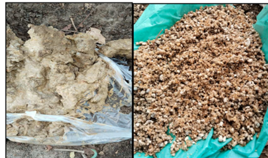
Fig. 16. Bore soil samples- yellowish white clay-0 to 19m & MCS-19-28m
