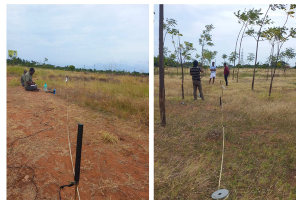
Fig. 6. D AMT scanning in the field with ADMT-300S model
