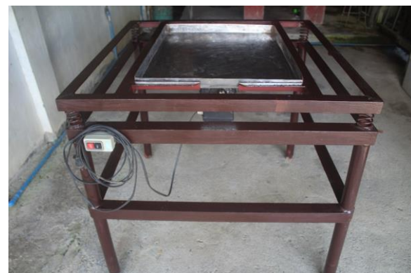
Fig. 3. Actual view of the chocolate bubbling machine
