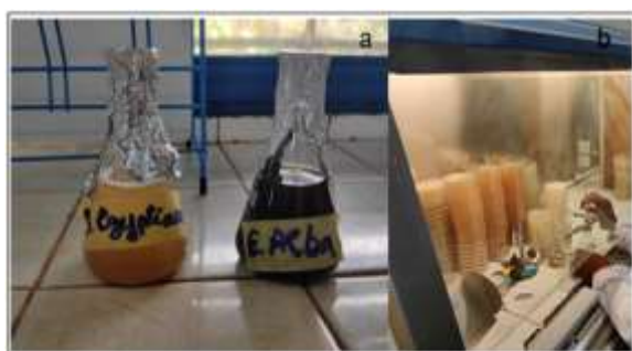
Fig. 2. Process of incorporating aqueous plant extracts into the PDA medium. (a) Aqueous extract before filtration; (b) filtration of extracts using Millipore filters.
