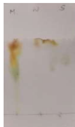
Fig. 2. TLC plate showed the various spots M-Methanol Extract, W-Water Extract, S-Standard
