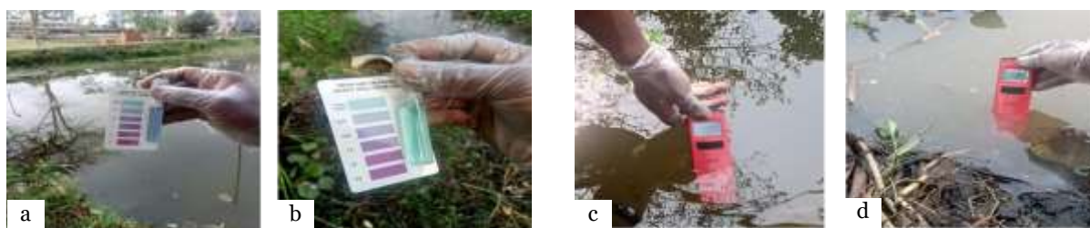
Fig. 3. (a) Ammonia measurement of pond 2; (b) Nitrate measurement of pond 3; (c) pH measurement on pond 2; (d) Measuring pH on pond 3
